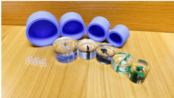
Samples mounted with high flow epoxy resin
